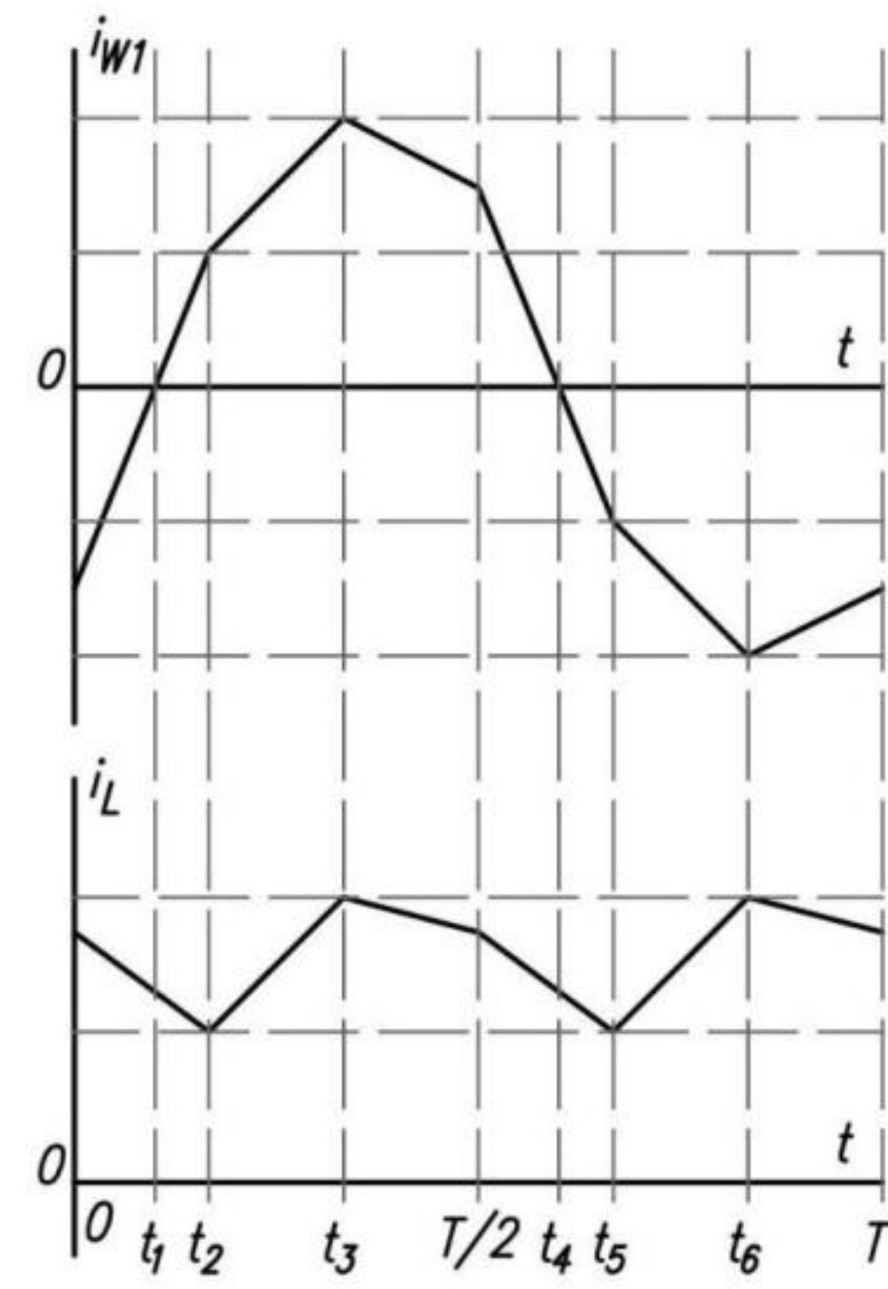
Fig. 3. The current of the primary winding i_{1w} of the TV1 and the current i_L of the L1 choke at PF-control
